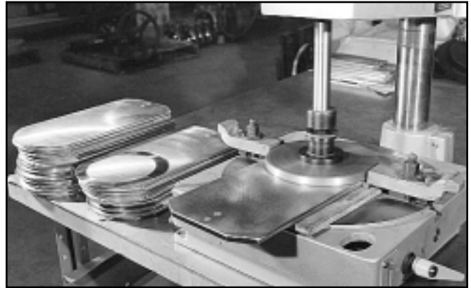
Figure 6.3B Knife Gate Lapping with a flat plate mounted on a drill press
