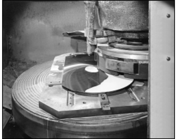
Figure 7.3C Grinding of entire knife gate surface with horizontal surface grinder
