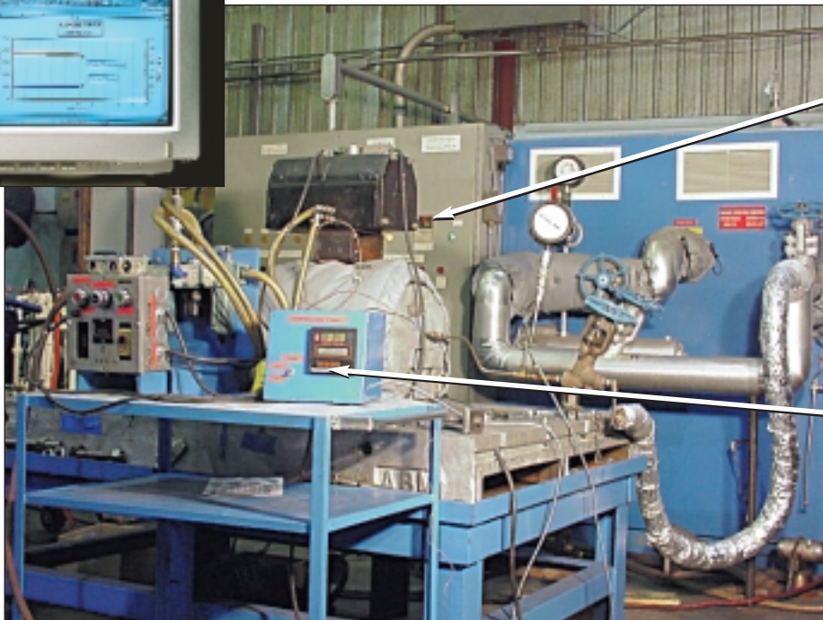
8" Class 300 valve hot cycled at 150 psi steam superheated to 800°F.
